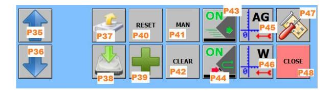
**P35 PROGRAM SCROLL UP:** this button scrolls up the programs list stored in the panel and recalls all the parameters and load it to the AG.
