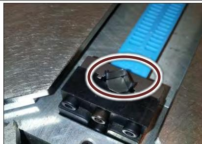
Use the tool to try to push down the wedge in the distribution head. The tool needs to be inserted only of about 5mm in the distribution head, then remove the tool and try to remove the cartridge.
