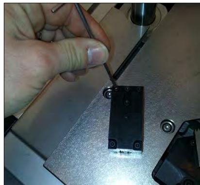
Separate the distributor plates and clean them using a clean cloth and lubricant spray.
