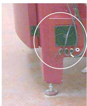
The NS has 3 DIN plugs to be connected to the machine, above the front right-hand foot.
