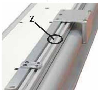
Unlock locking screw Z and slide the guide GB of the NS along screws 1-2-3 of the right-hand table and the nuts of the 2 ruler supports R1 and R2. Screw 3 should be visible in hole T3. Tighten screws 1, 2, 3 and V1 and V2 of ruler supports R1 and R2 with a 4mm hex head key.
