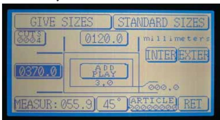
The file parameters displayed in this screen are the last parameters created, modified, listed or executed. This means that after a machine power failure, you do not need to re-enter a reference before resuming work. Also, you can list the file that you are interested in and then execute it without having to call up its reference.
