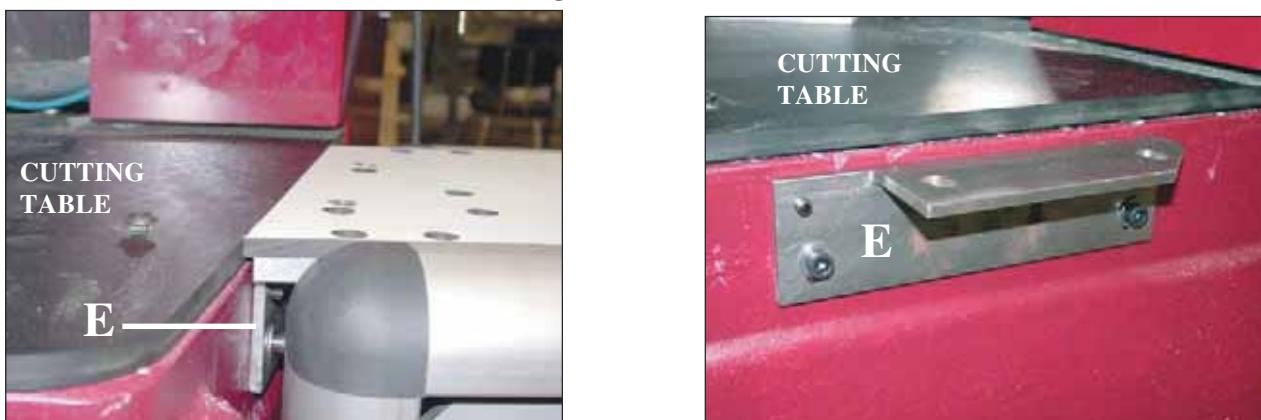
Take the NS out of the crate and turn it over. Place the bed of the NS on bracket E, and screw them together (10mm long tubular socket wrench + 5mm hex head key) without tightening, with the 2 screws, 2 washers and 2 nuts provided.
